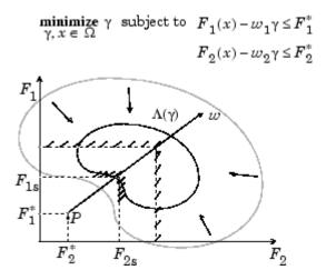
Figure 3-12: Geometrical Representation of the Goal Attainment Method
