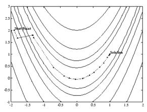
Figure 3-4: Levenberg-Marquardt Method on Rosenbrock's Function
