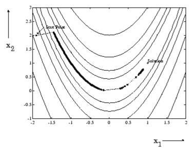
Figure 3-1: Steepest Descent Method on Rosenbrock's Function (Eq. 3-2)
