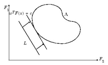
Figure 3-9: Geometrical Representation of the Weighted Sum Method
