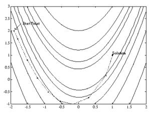
Figure 3-3: Gauss-Newton Method on Rosenbrock's Function
