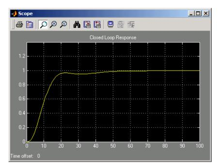
**Closed-Loop Response Using fminimax**
