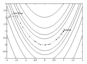
Figure 3-2: BFGS Method on Rosenbrock's Function
